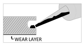
Make sure glue is applied in a continuous line (3/32" to 1/8" bead) otherwise your floor will squeak. Clean excess glue immediately with a damp cloth followed by a dry cloth. Adhesive allowed to dry on board surface will be difficult to remove and may leave a haze.
